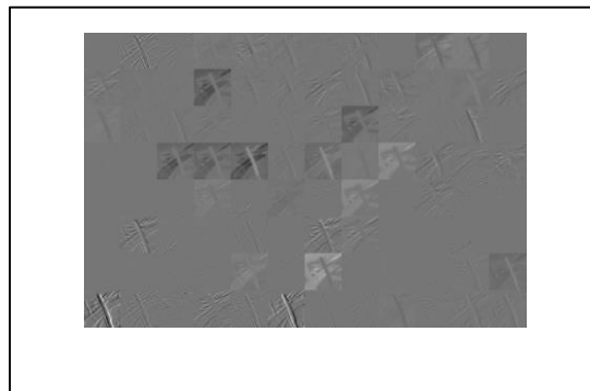
Figure 4. Activations / Feature maps in All Channels of Convolution Layer 1 for the Test Image in Figure 3.
